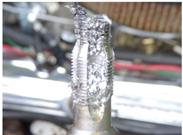
"...if you load the tap up with a lot of grease, the chips...stick to it and [don't] fall into the cylinder ..." (photo by the author)
