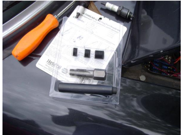
"...so I thought I would get a helicoil and was able to find one at NAPA .." (photo by the author)
