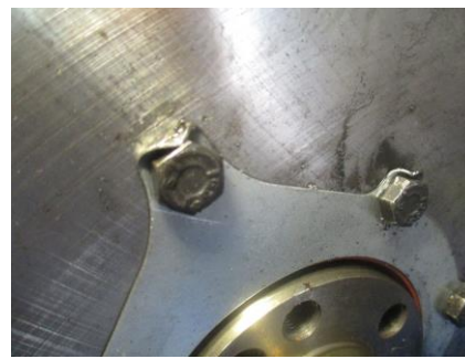
"62. Un-bent tabs on rear main seal retainer.... See picture #26..."
