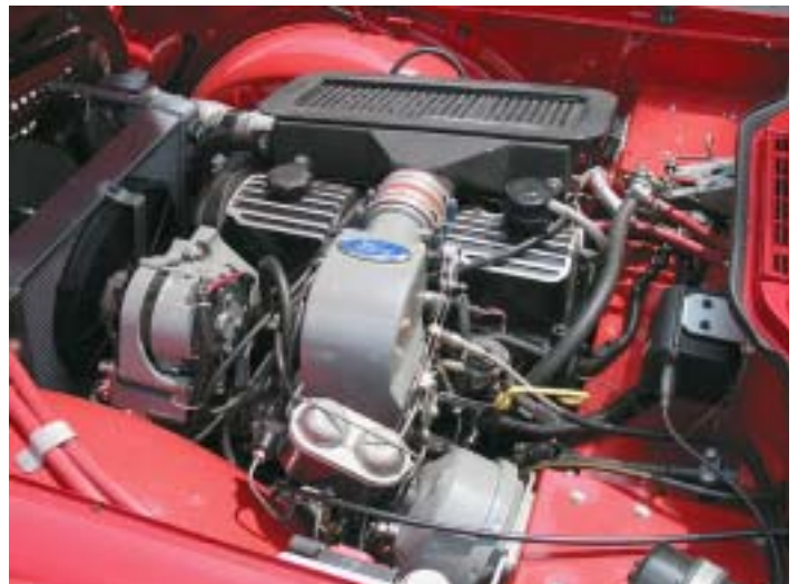
TR6 with 4 cylinder turbocharged Ford and big tires
