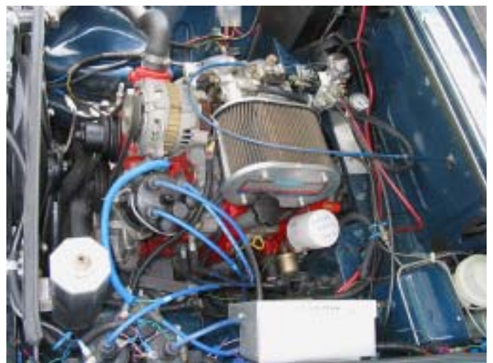
MGB with Mazda RX7 rotary engine
