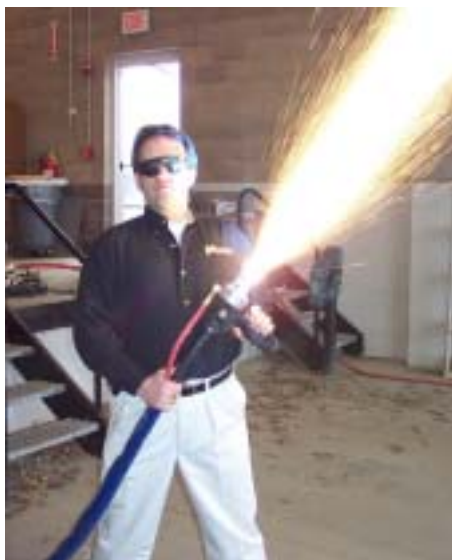
Twin Arc Plasma Spray in Action
