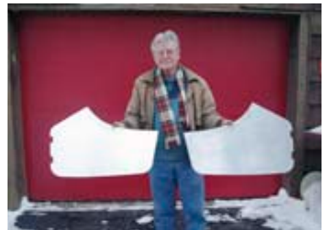
Ron Lindemann, reskinned the doors in aluminum
