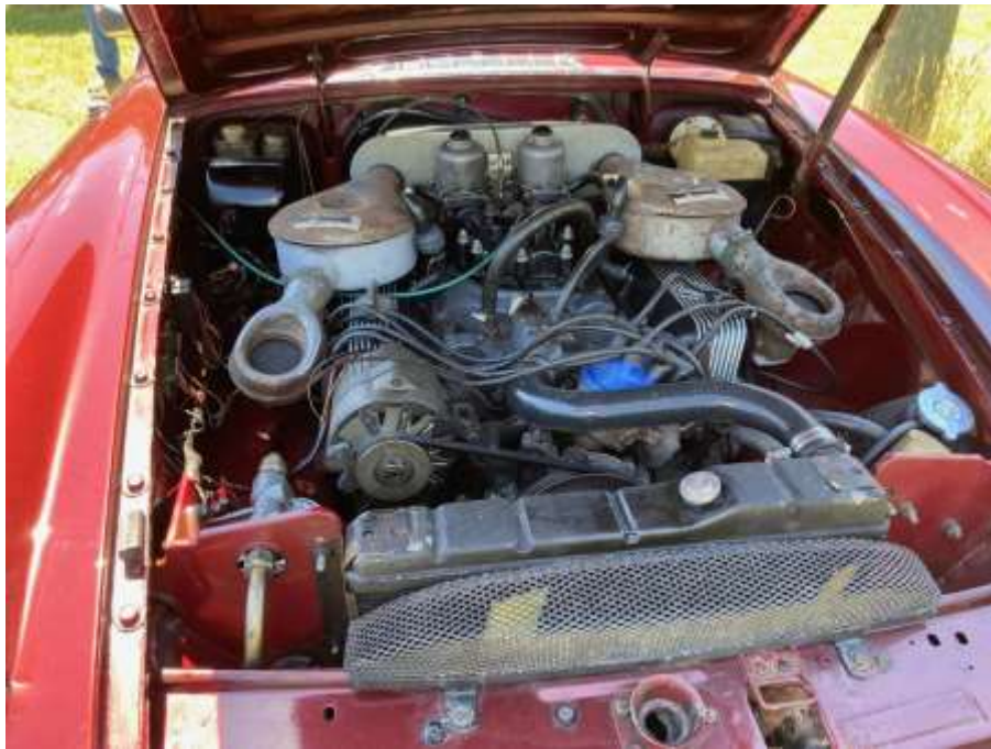
A look at the engine compartment of a factory 1974 BGT V8. Note the unusual air filter/carbs/intake arrangement to keep most of that hardware towards the back of the engine and avoid the need for a bonnet bulge.
