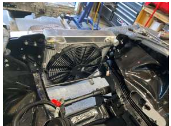
Radiator and fan are mocked up and ready for final install when the engine is in for good.
