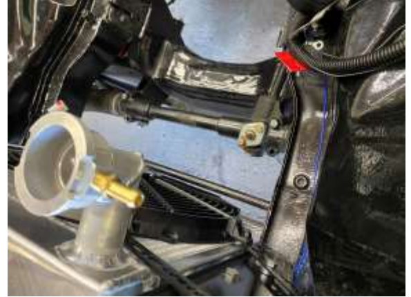
Now the fan clears the front sway bar, and the radiator sits 1" lower in the car so the filler neck clears the hood.
