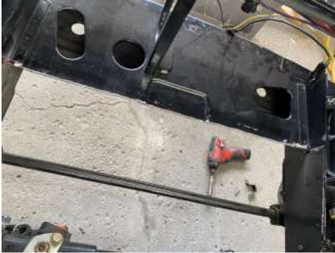
This is the panel I removed 1/2" of material from to gain the needed clearance to move the radiator forward.
