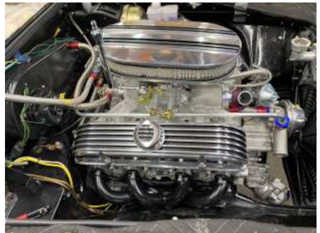
The long coolant tube for the heater was installed. This is a nice unit from D&D which looks much better than draping a hose all the way to the water pump. I modified a finishing clamp to give the appearance of an AN fitting. You'll notice there is a short hose that goes between the water pump and intake manifold. Murphy's Law states that the hose with the greatest chance of leaking will be the one that's hardest to get to, and this hose followed that law to the letter. I had to remove the intake manifold, install a beefier clamp in the AN style finishing clamps, and retighten the clamps. It worked the second time. The chrome fuel line sticking straight up could not be used, as it reached all the way back to the heater fan. I switched it out to a standard banjo fitting.
