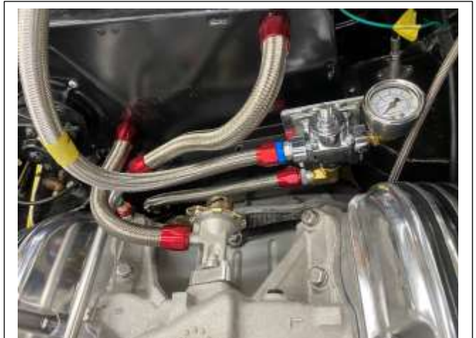
Heater hoses and fittings are installed. As I stated earlier, I've never used stainless hoses before so I wasn't sure what to expect. The finishing clamps also has some pretty anemic looking clamps, so I was a bit apprehensive they would hold.
