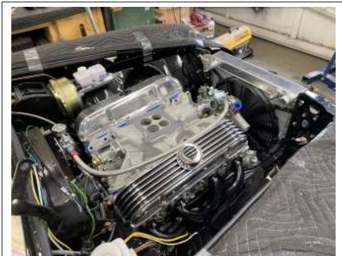
First items to go on are the valve covers, mainly to keep dirt and crud from finding their way into the engine. The fuel line from the regulator to the carb is fitted but not cut to length yet.
