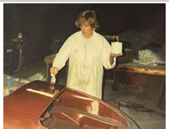
Painting protective primer
